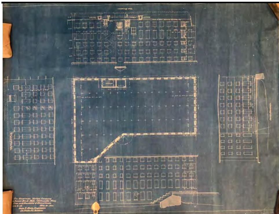
Figure 8 1900 blueprints for Butterworth Building, showing the five-story building. Dean & Main, engineers, American Woolen Company, Beaver Brook Mill Storage Building, Dracut, MA, plans, and elevations, (1900) Mass. Dept of Public Safety Records, #6327, Massachusetts Archives.
