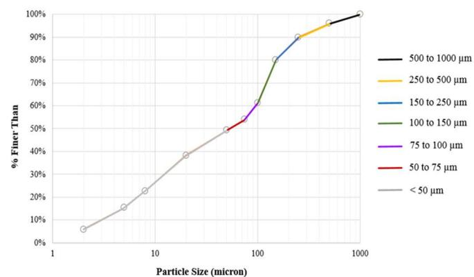
Figure 2 - Particle Size Distribution of Test Sediment
