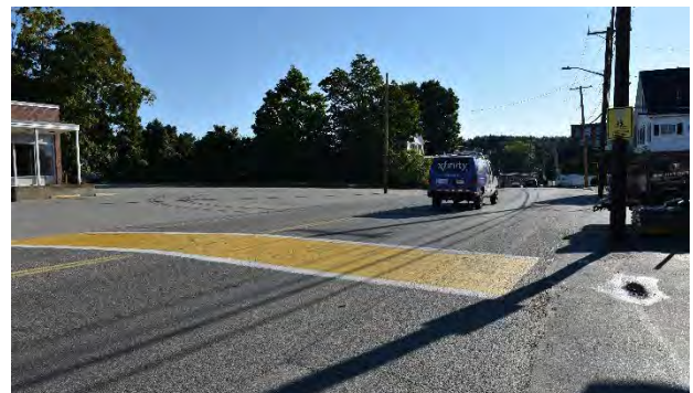
Figure 7. Midblock crosswalk not connected to sidewalks on either side of Lakeview Avenue. A non-MUTCD compliant crosswalk warning sign.
